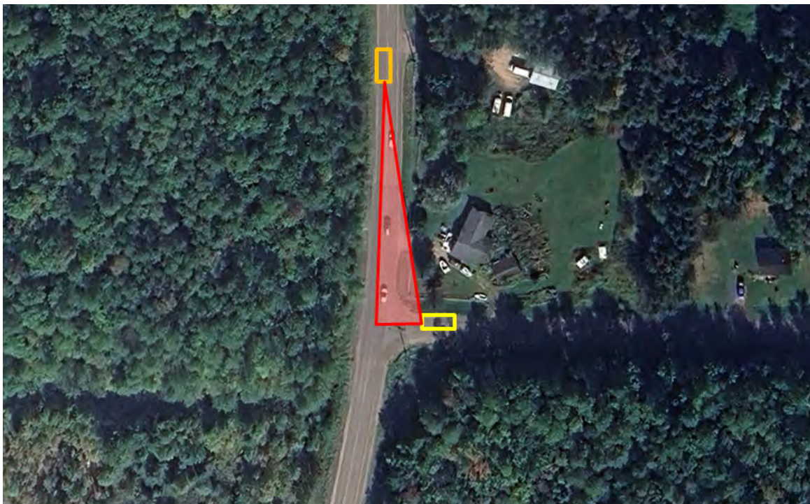
Figure 12 | Intersection Sight Distance Sight Triangle Example at Bishop Lane and Blueberry Road 25 mph Operating Speed Assumed (Google Earth)
