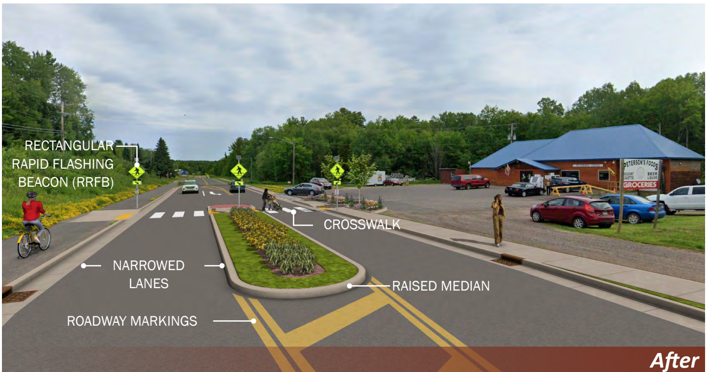
Figure 55 | Proposed improvements at Peterson's Crossing aim to enhance visibility and safety for pedestrians and cyclists through the addition of roadway markings, a raised center median, curb cuts, and increased signage. (Terra Soma)
